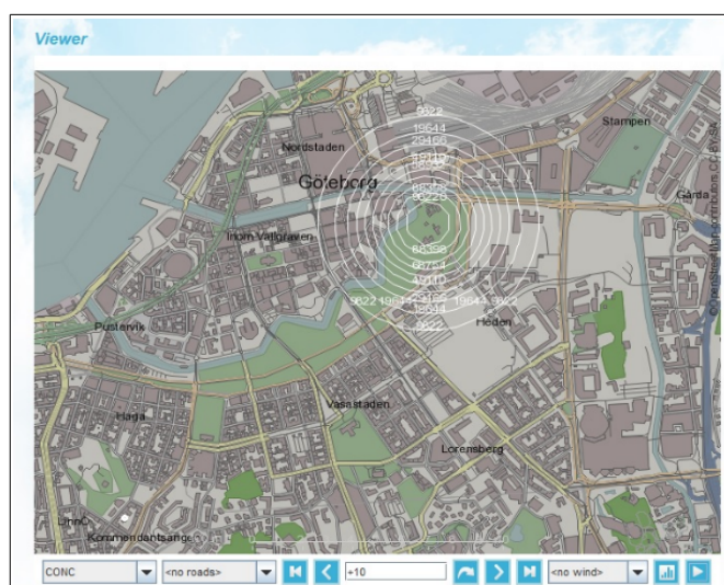
Figure 2.5.3 Ammonia leakage from a tank burst, 10 minutes after the burst.
