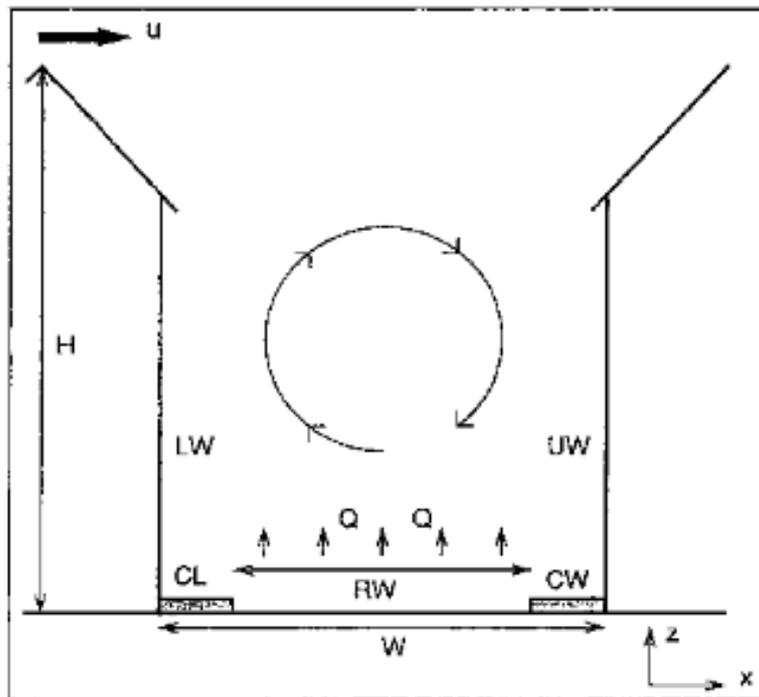
Figure 2E.1 Principles of air circulation within a street canyon (the upwind side is denoted UW, the leeward side LW, see also notations for house height ( $H$ ), street width between houses ( $W$ ) and road width ( $RW$ )).
