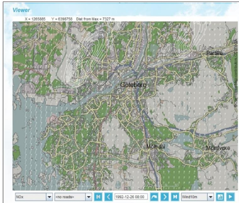
Figure 2.4.2 The two NO<sub>x</sub> plumes and the wind field at 921226 08 and 921226 12
