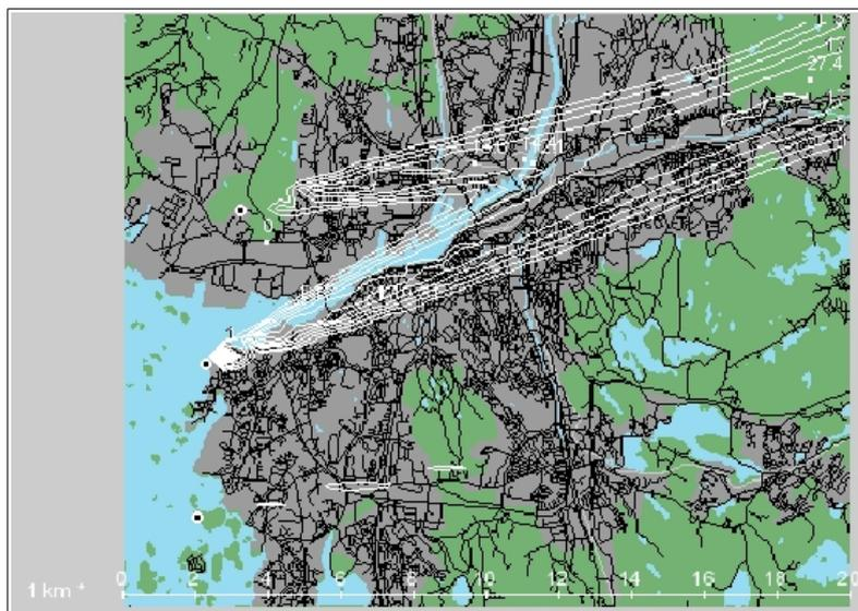
*Figure 2.2.2.7 Three stacks with a 2.5 m/s SW wind.*
