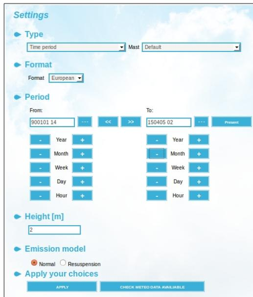
Figure 2.7.1. Aermod. Model Settings
