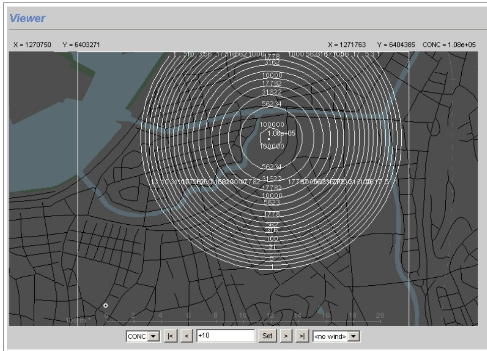
Figure 2.5.3 Ammonia leakage from a tank burst, 10 minutes after the burst.
